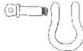
Screw-Pin Clevis: Attachment hardware for use with larger pull blades. \frac{7}{16} ", \frac{1}{2} ", \frac{3}{4} ", 1".
